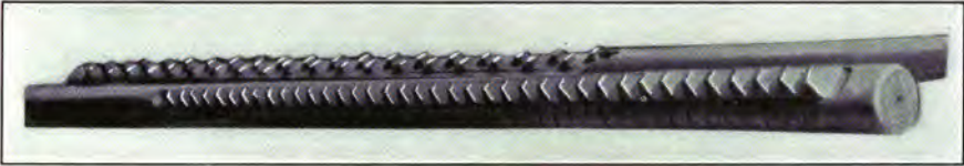
FIG. 142.—Two inserted-tooth broaches.
